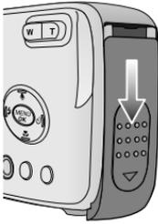
1. Open the battery chamber cover by pushing in the direction of the arrow.
